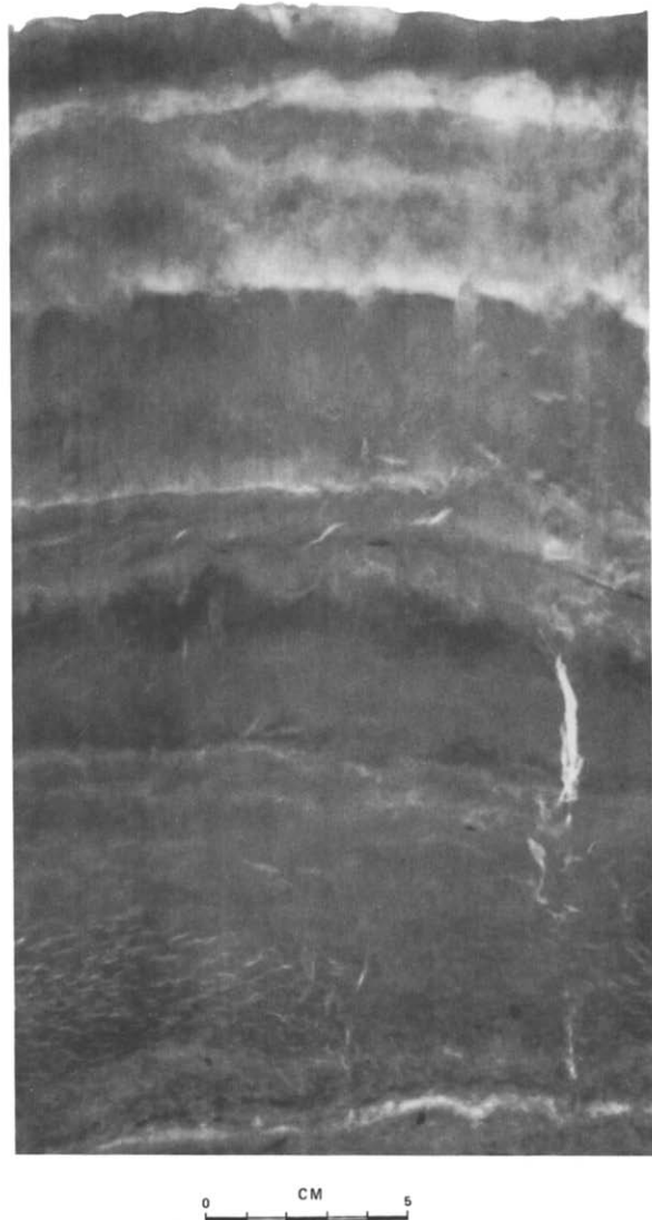
Fig. 3. Representative X-radiograph of sediment collected in 1980. The depth scale is compressed due to sediment desiccation.
